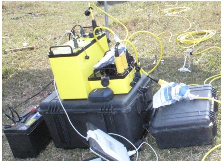
Figure 3.5. SuperSting R8/IP system with 56 electrodes and Switch box connection for IMEE data acquisition
