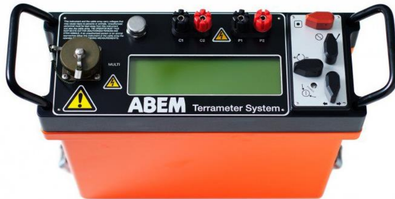
Figure 3.8. ABEM Terrameter SAS 1000 for 2D ERT data acquisition
